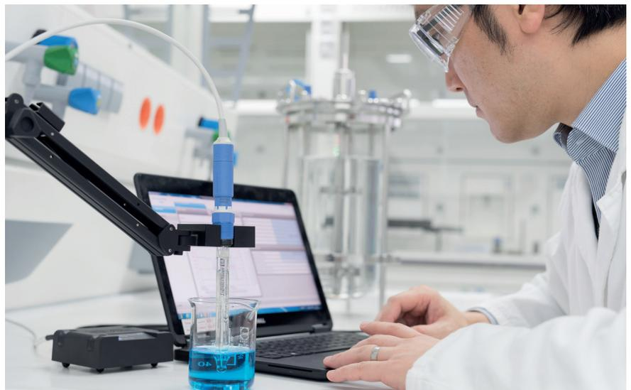
A crucial activity during fermentation is the control of the acidity of the culture medium which is measured by the indispensable pH sensor.
