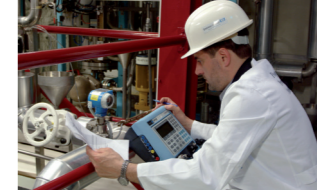
On-site calibration of pressure devices
